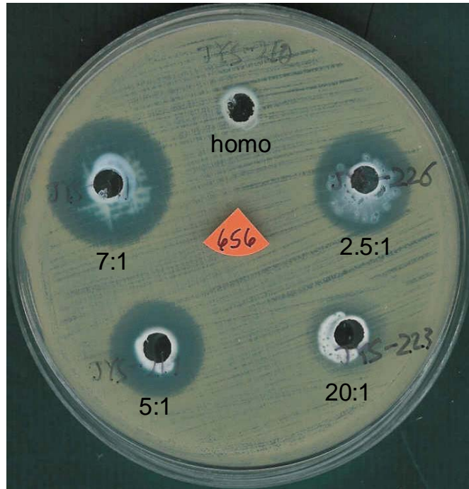
Fig. 3-23 Antibacterial testing of drug-embedded nanoparticles against MRSA 656 (ratios of ethyl acrylate : lactam indicated)
